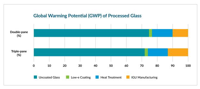
Of the embodied carbon in an IGU, approximately 75% comes from manufacturing the flat glass lites. Of the remaining, 13% comes from heat strengthening or tempering the glass, 10% comes from the IGU fabrication process itself, and just 2% comes from the process of adding low-e coatings.
